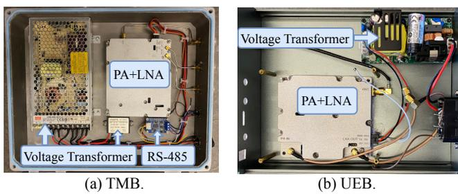
Fig. 3: Internal view of TMB and UEB.
