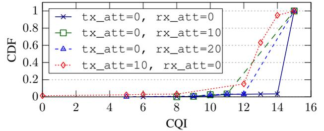
Fig. 6: CQI variation for different attenuation levels.
